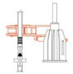
Grip on Hard Facing Not recommended Reduces lifespan of Jaws/Bits Breakout Action Not Reliable
