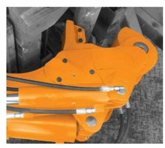
The Mammoth Breakout Wrench fitted to a DM30II/ CDM30 Rig
